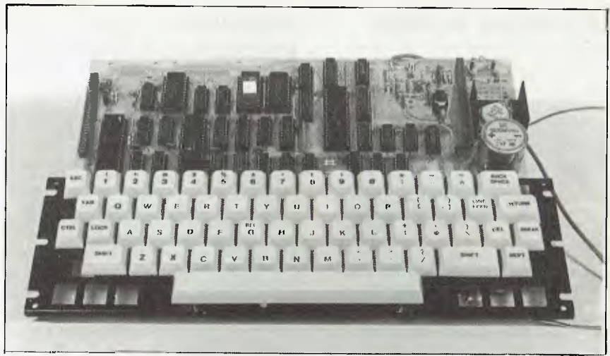
MicroBee with cover and coreboard removed.
